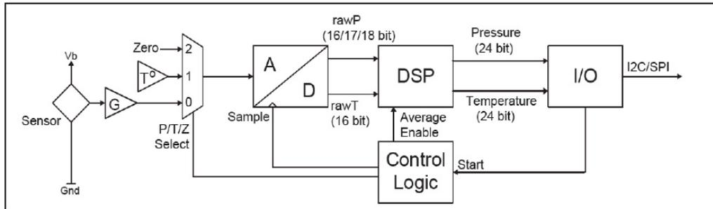
The ADC performs conversions on the raw sensor signal (P), the temperature reference (T) and a zero reference (Z) during the ADC measurement cycle.
